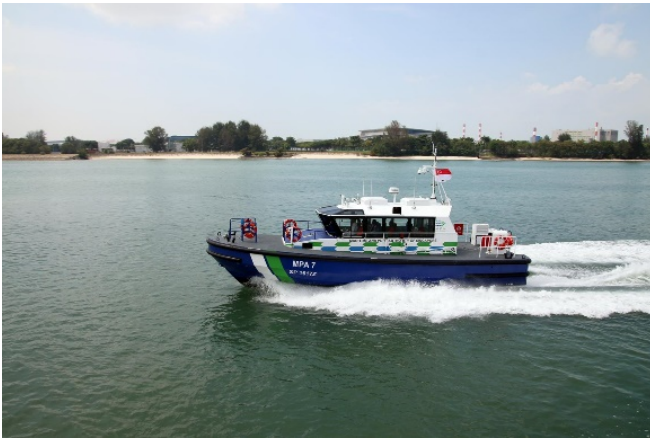
The 15-metre pilot boat, built by Lita Ocean for the Maritime & Port Authority, is powered by two Scania DI13M engines
