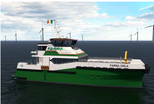
The 27-metre wind farm vessel, built by Penguin International to the Incat Crowther 27 design, is powered by quad Scania DI16 077M engines
